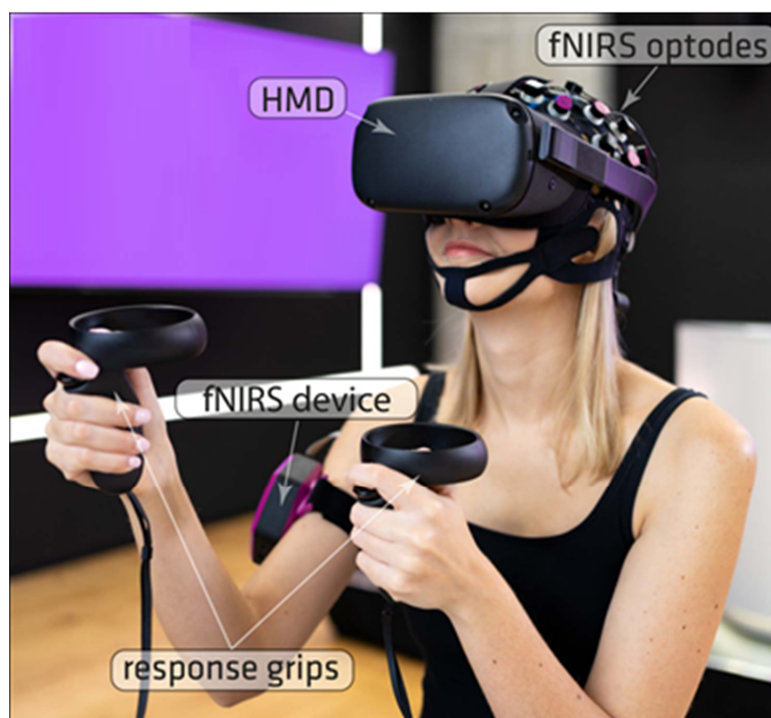
Figure 1. The experimental setup included wireless all-in-one VR goggles and a wearable fNIRS device. Participants were seated during data recording and the devices were not connected by a cable.
