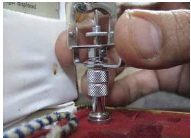
Fig. 2: Checking Schiotz tonometer for zero error
