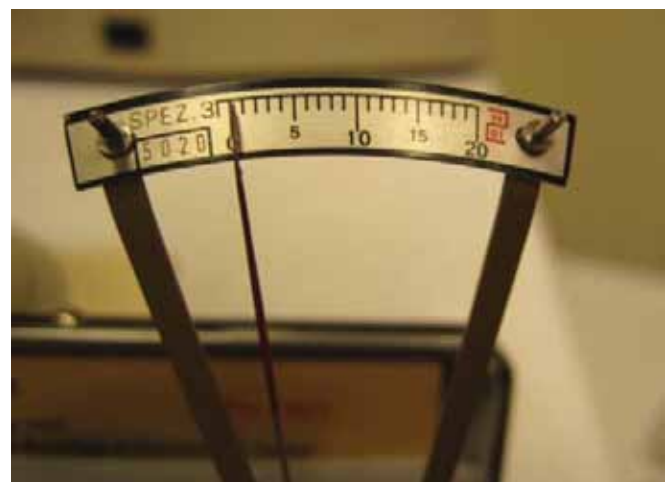
Fig. 3: Checking the Schiotz tonometer on a dummy cornea before use
