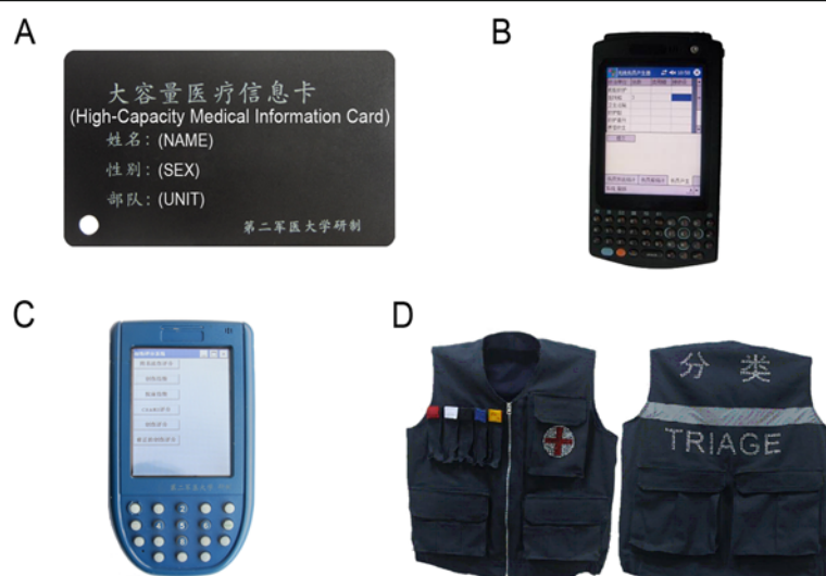
Figure 1 Four components of triage and medical evacuation system for casualties at sea. (A) The high-capacity medical information card, which has an RFID chip inside and a PVC plastic shell outside, can identify wounds, track casualties through triage process and transmit information to institutions at all levels. (B) The simulated patient generator can provide specific types of casualties for the simulation training of medical personnel, which increases the training intensity and improves the rescue abilities of medical personnel. (C) The Triage classifier can capture the casualties' information, generate the trauma index and conduct the casualty triage, which can guide medical personnel in providing first aid to the wounded and performing medical evacuations. (D) The multifunctional airbag triage vest is composed of an airbag device, a multipocket design and fluorescent strips, and it is capable of carrying colored markers and other medical instruments. Red tags indicate hemorrhage, White tags indicate fracture, Black tags indicate infectious disease, Blue tags indicate radiation disease and Yellow tags indicate biological agents.
