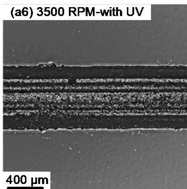
(b) SEM images of the bottom of the surface micro-machined regions
