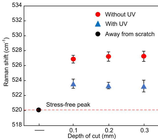
Fig. 14. The effects of depth of cut and ultrasonic vibration on Raman peak position.
