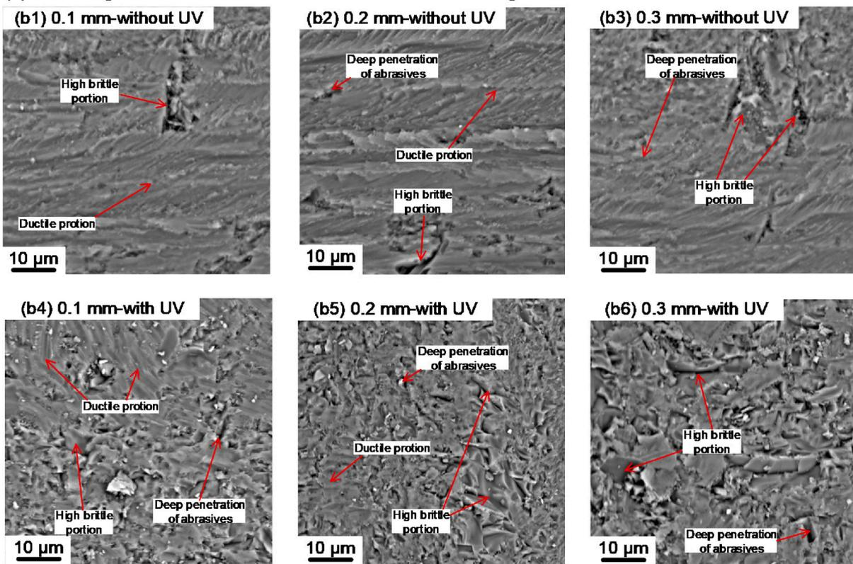
Fig. 13. Effects of the depth of cut on cutting surface morphology with and without ultrasonic vibration: (a) the OM images of the contour of the surface micro-machined regions and (b) the SEM images of the bottom of the surface micro-machined regions.
