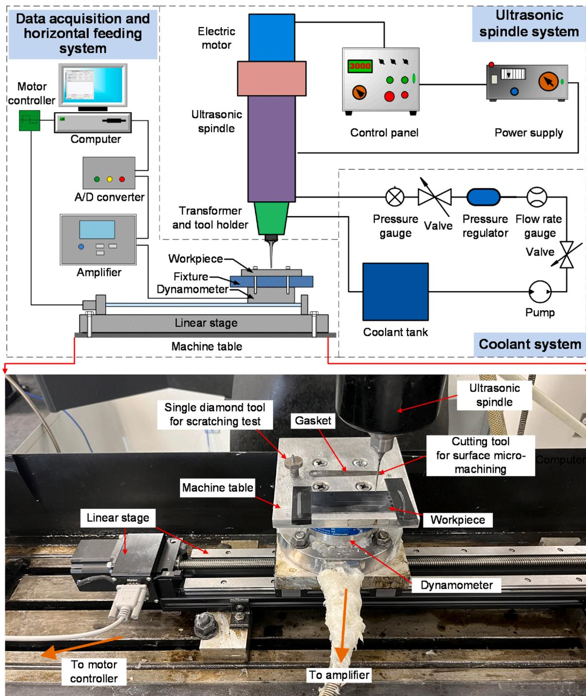
Fig. 1. The illustration and photograph of the experimental setup for the rotary ultrasonic micro-machining (RUS $\mu$ M) process.
