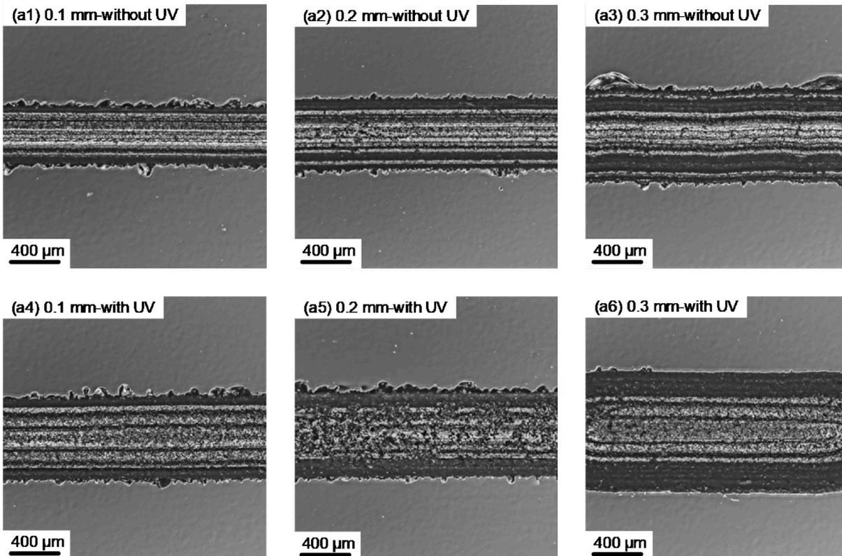
(b) SEM images of the bottom of the surface micro-machined regions
