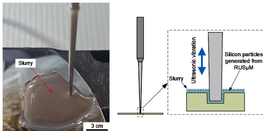
Fig. 7. The illustrations of ultrasonic machining (USM) mechanisms in the rotary ultrasonic surface micro-machining (RUS $\mu$ M) process.
