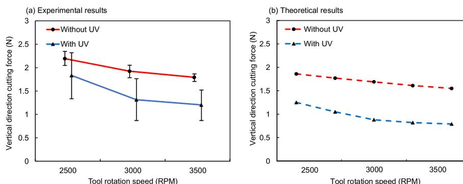
Fig. 8. Effects of the tool rotation speed and ultrasonic vibration on the vertical direction cutting force: (a) experimental results and (b) theoretical results.
