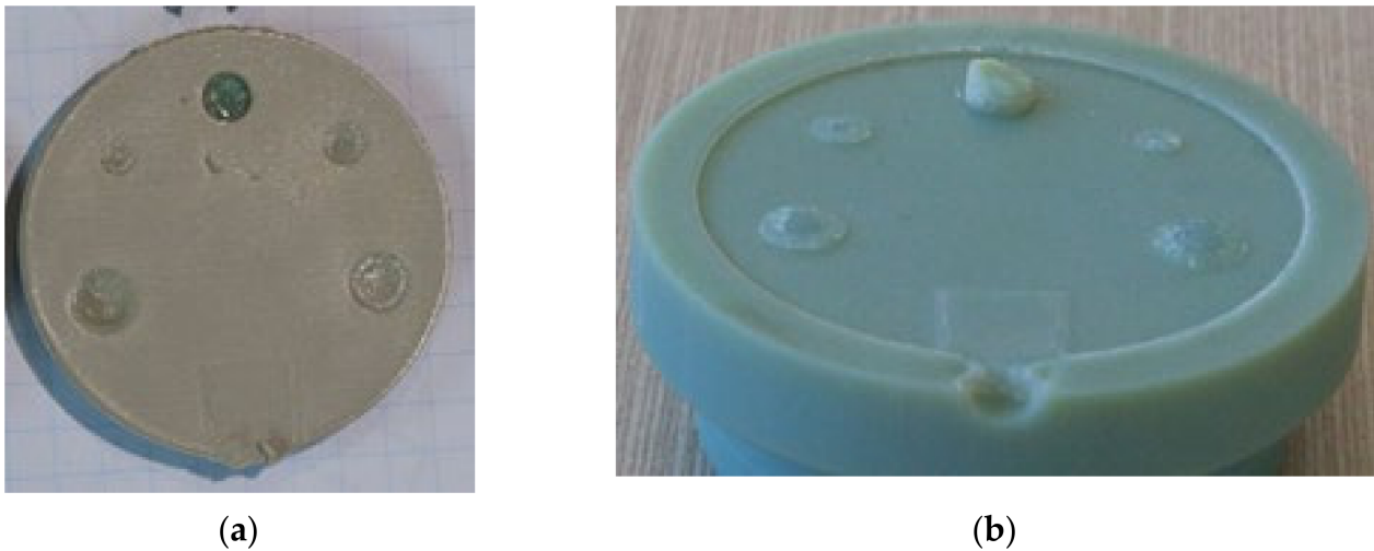
Figure 29. (a) 12th moulded part showing defects (b) State of core pins (broken) on the 3DIM after 12 shots. The moulded parts have no cored holes as the core pins on the tool are completely broken.
