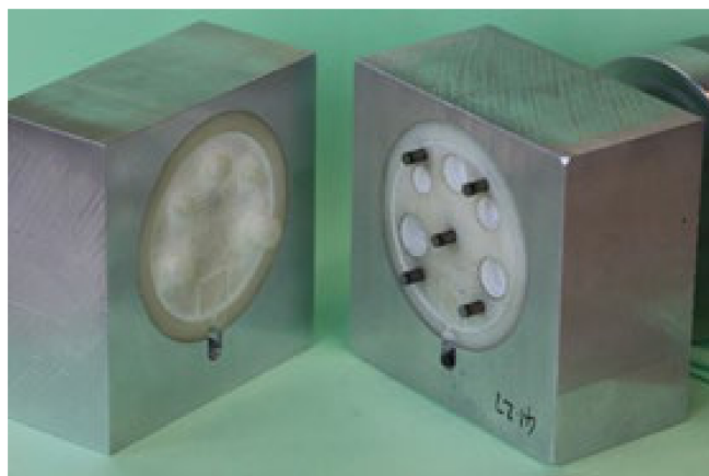
Figure 4. Core and cavity 3DIM inserts assembled inside a MUD base along with ejector pin assembly. The white parts are the 3DIM tools and the aluminium housings are the MUD base.
