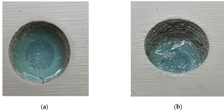
Figure 26. (a) Top view of M5 core on pin 6th part showing a small chunk of green 3DIM material of core pin stuck inside; (b) orthographic view of M5 core hole on 6th part showing a small chunk of green 3DIM material of core pin stuck inside.
