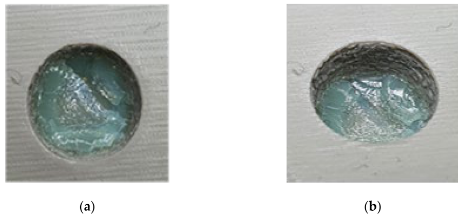
Figure 27. (a) Top view of M5 core on pin 8th part showing a small chunk of green 3DIM material of core pin stuck inside; (b) orthographic view of M5 core hole on 8th part showing a small chunk of green 3DIM material of core pin stuck inside.
