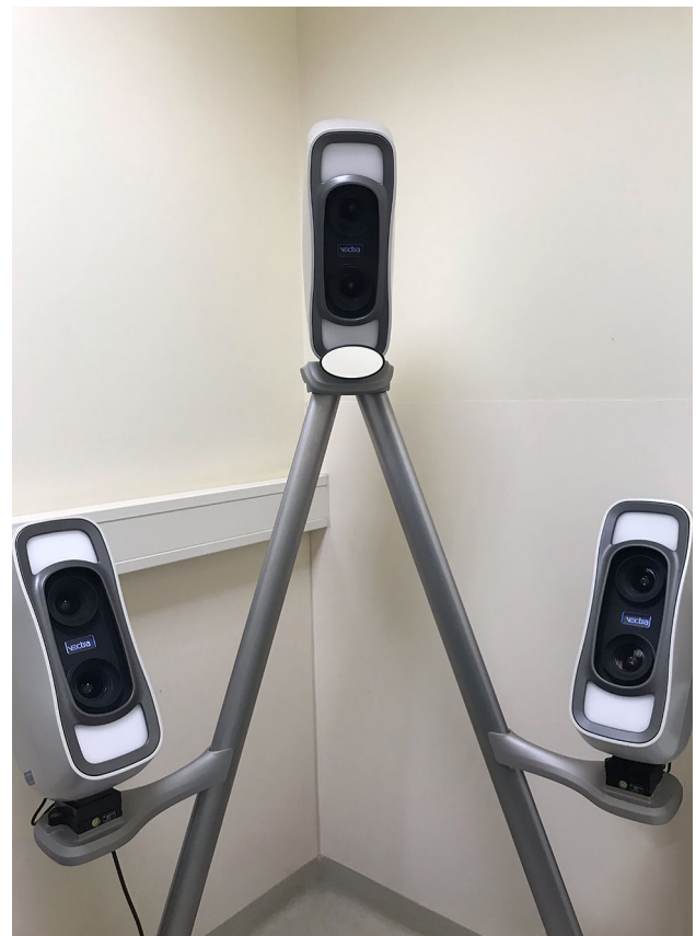
Fig. 3 VECTRA M3 system used for Stereophotogrammetry analyses.
