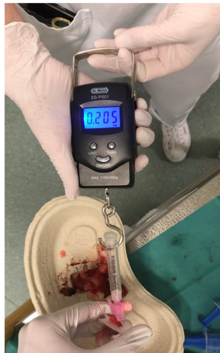
Figure 4. An electronic spring scale was connected to a prepared disposable syringe and to the catheter via a Luer lock connection. By slowly pulling the disposable umbilical clamp, the force to release the securement was measured.
