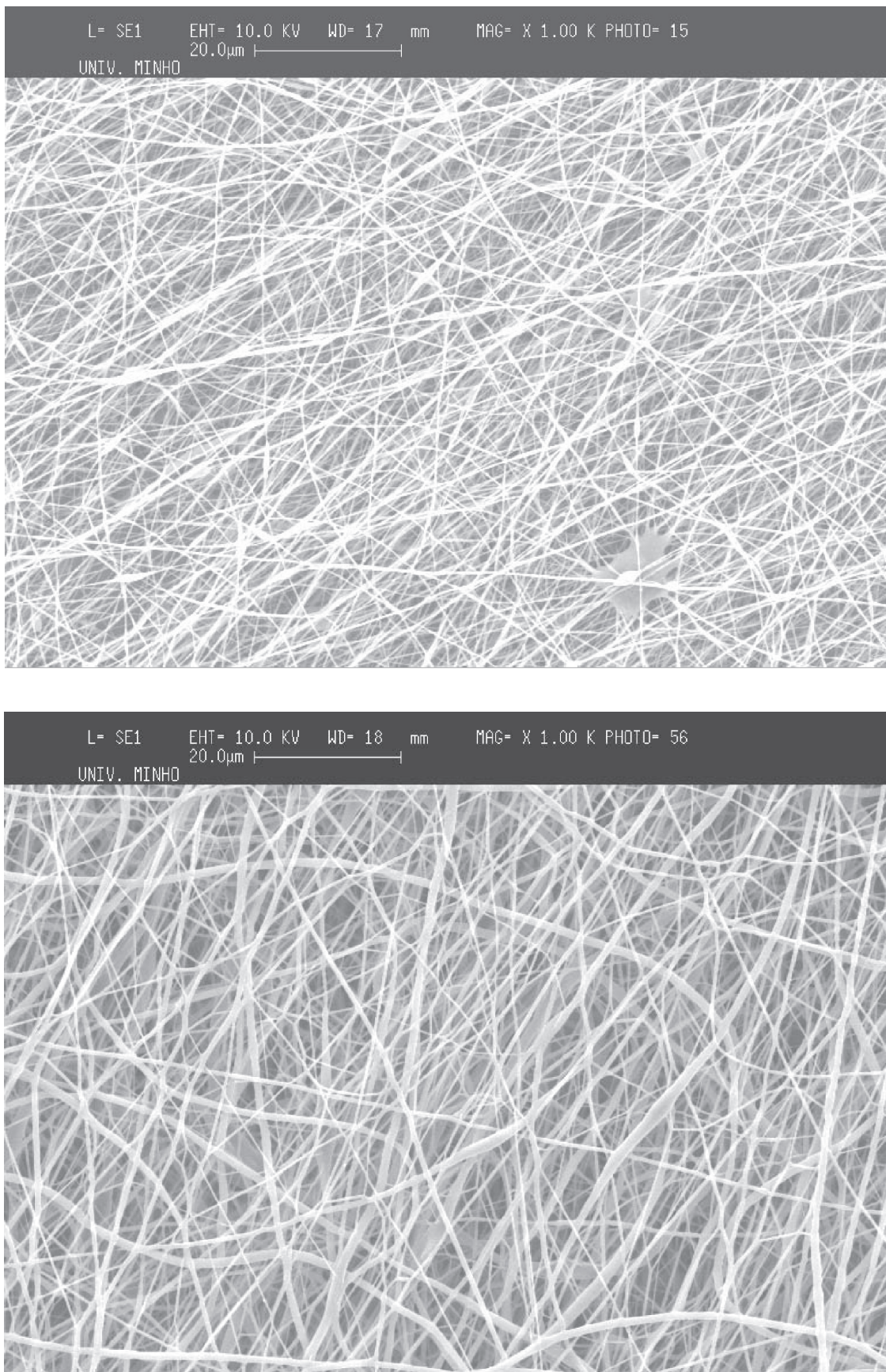
Figure 3 SEM micrographs of meshes obtained with PEO (top) and PCL (bottom) with similar deposition time.
