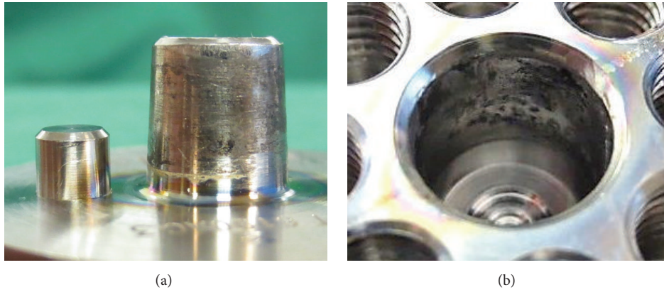
FIGURE 3: Severe tribocorrosion on male (a) and female (b) taper of a retrieved prosthesis. The time to revision was 9.2 years.
