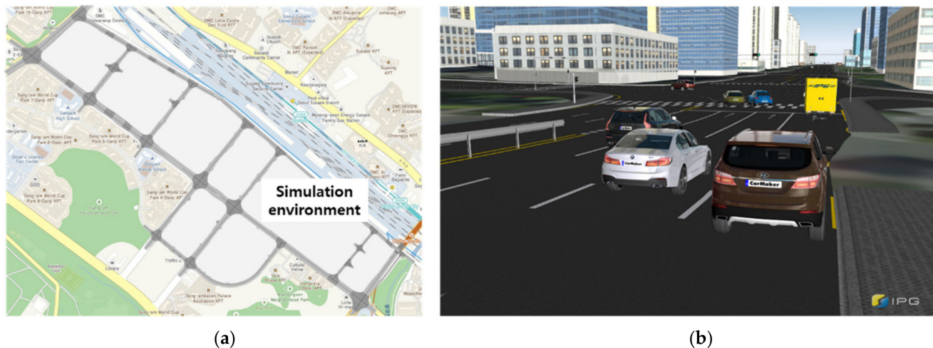
Figure 10. Virtual test-driving environment based on real road data: (a) simulation environment and (b) virtual driving scene.
