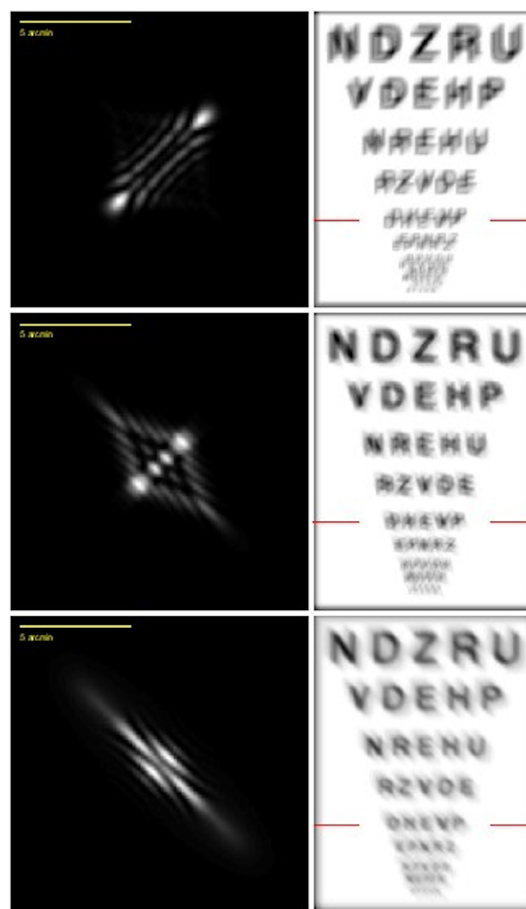
FIGURE 1 Example of multiple point spread function (PSF) cores inducing polyopia. PSFs (left column) and computed retinal images (right column). Model wavefront aberration was W = C_2^0 Z_2^0 + 0.4 Z_2^{-2} + 0.1 Z_4^0 , for three values of additional defocus: C_2^0 = -0.3 \mu\text{m} (top row), C_2^0 = 0 \mu\text{m} (middle row); and C_2^0 = +0.3 \mu\text{m} (bottom row). Pupil diameter = 6 mm. Red line identified the 0.0 logMAR letter size.
