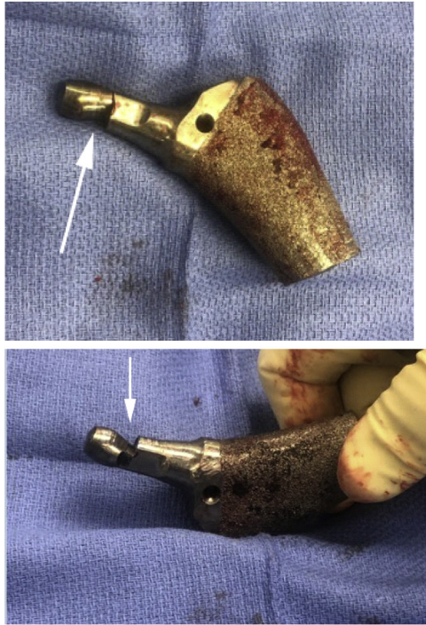
Figure 3. Explanted femoral stem demonstrating erosion of the proximal portion of the taper and a half-thickness crevice (arrows) in the femoral neck.
