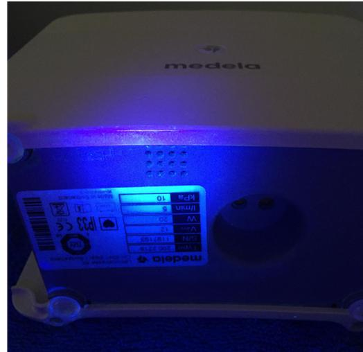
**Figure 4.** No evidence of aerosolisation from the exhaust holes of the DD-CDS at maximum settings (300 mL of fluid level and 5 L/min of air leak volume). The canister is removed as the drainage system is tilted over.
