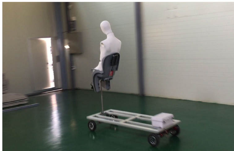
Figure 13. Motorcar with a mannequin for collision testing.
