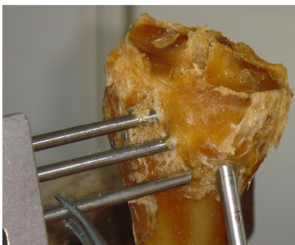
Fig. 2 When the rotation angle of the guide is greater than 60°, less bone is penetrated through the sleeve of the cross pins and more is exposed
