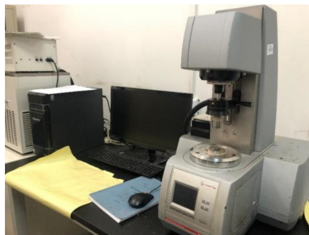
Figure 5. Dynamic shear rheometer (DSR) equipment consists of a temperature control system, a stress and strain control system, and an automatic data analysis system.
