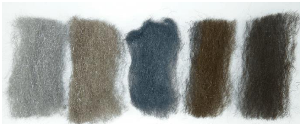
Figure 2. Wool samples after thermal treatment under an inert atmosphere. From left to right: Initial sample, sample treated at 200 °C, sample treated at 300 °C, sample treated at 400 °C, and sample treated at 500 °C.
