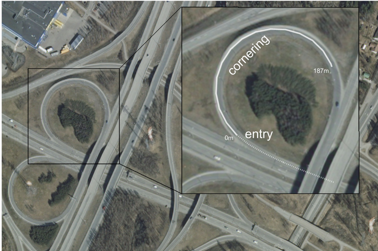
Figure 2. The motorway on-ramp used in the study (Kehä III - Lahdenväylä, N 60.274643; E25.086422). Inset: the entry (dotted line) and cornering (solid line) phases of the curve, based on GPS data from an individual run. For explanation of sequencing the curve see main text. The cornering phase is 187 m in length. Image source: National Land Survey of Finland open Topographic Database. license version 1.0 -1 May 2012.
