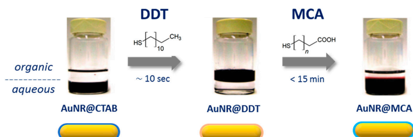
Figure 17. Round-trip" phase transfer method to prepare a DNA-AuNR bioconjugate [153].
