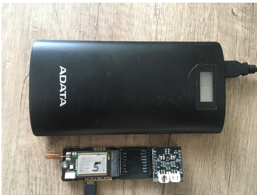
Figure 11. Mobile measuring system composed of modular sensor and power bank.
