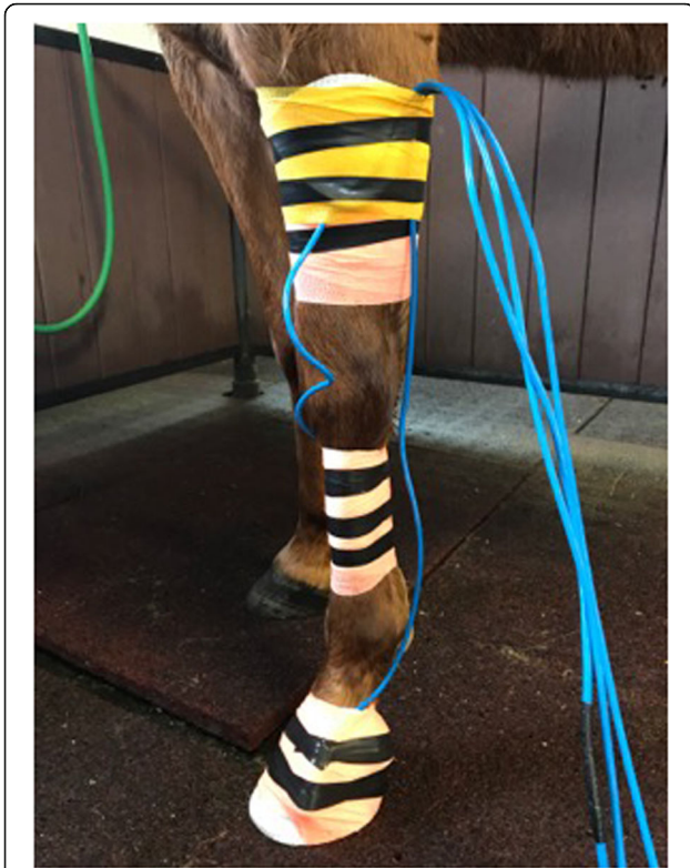
Fig. 4 Application of three uniaxial, water submersible accelerometers to the left equine forelimb. Accelerometers are secured at the hoof (lateral), mid cannon (medial), and mid radius (medial) with adhesive wraps
