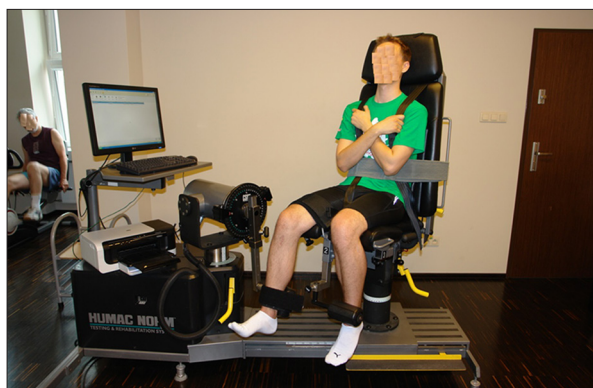
Figure 6. The starting position of the torque measurements of knee extensors and flexors under isokinetic conditions.
