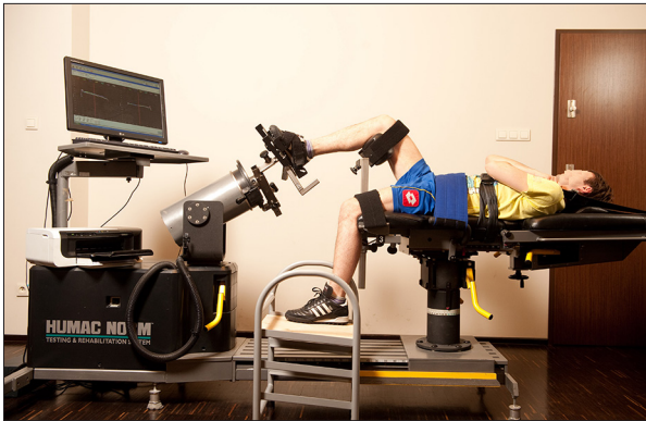
Figure 2. The starting position of the torque measurement of muscles responsible for internal and external shin rotation in the knee joint and the starting position of the training of muscles internally rotating shin towards femur in the operated knee joint on the Humac Norm Testing and Rehabilitation System.
