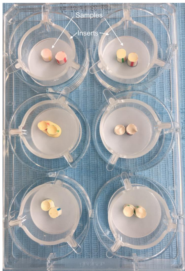
Figure 2. Fresh and set samples transferred into inserts, separating the sealer and establishing indirect contact with the material and the cells
