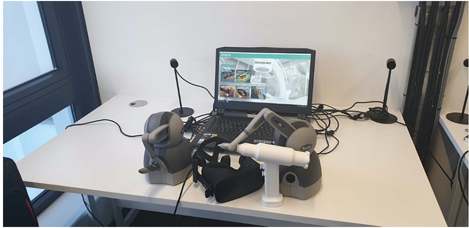
FIGURE 1: Virtual reality tool including a display device, headset and haptic devices
