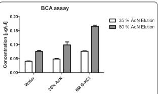
Figure 2 Polypeptide concentration in the ultrafiltrates eluted with 35% and 80% AcN following C18-SPE desalting. Each
