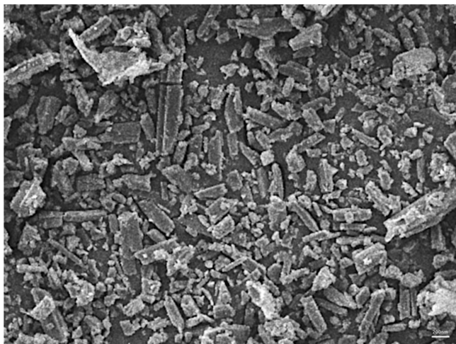
Figure 7. SEM image showed rod shape nanoparticles of NSE4 formulation.
