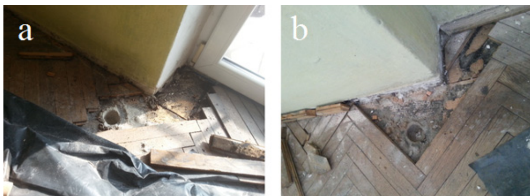
Figure 3. Floor material sampling points in two different (a) and (b) residential buildings (photos taken by the authors).
