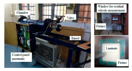
Figure 3. Gas gun experimental set-up used for impact testing on the composite laminates.
