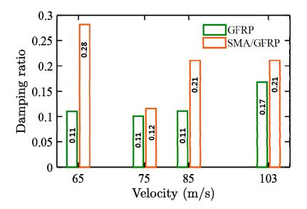
**Figure 10.** Damping ratio vs. velocity response for the GFRP and SMA/GFRP specimens at different impact velocities.
