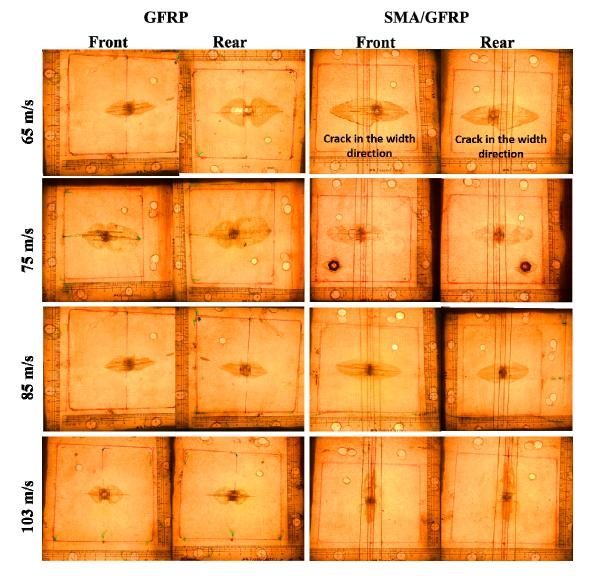
be seen in Figure 6. The cracks were originated from the primary region and extended in the width direction transverse to the aligned SMA.
