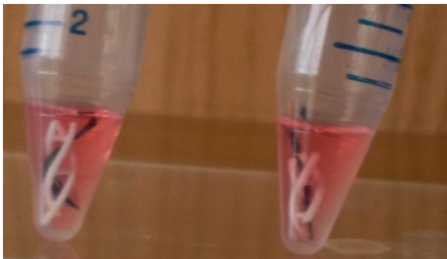
Figure 3. 3D-printed lattices with embedded–knitted carbon fibers during the cell culture process.
