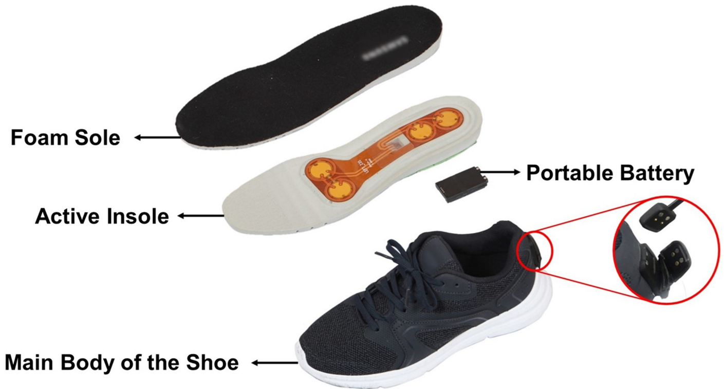
Fig 1. The custom-built shoe with an active insole. The system consisted of a foam sole, an active insole, a portable battery, and the main body. The portable battery could be attached to the bottom of the active insole. Mechanical vibration was applied to the metatarsal head and heel using the actuators in the active insole, which could be placed inside the shoes and connected to the charging port of the shoes. The red circle shows a magnified view of the charging port that can be opened and connected to a custom-made power cable.
