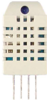
Fig. 3. The DHT22 sensor that can measure both temperature and humidity.
