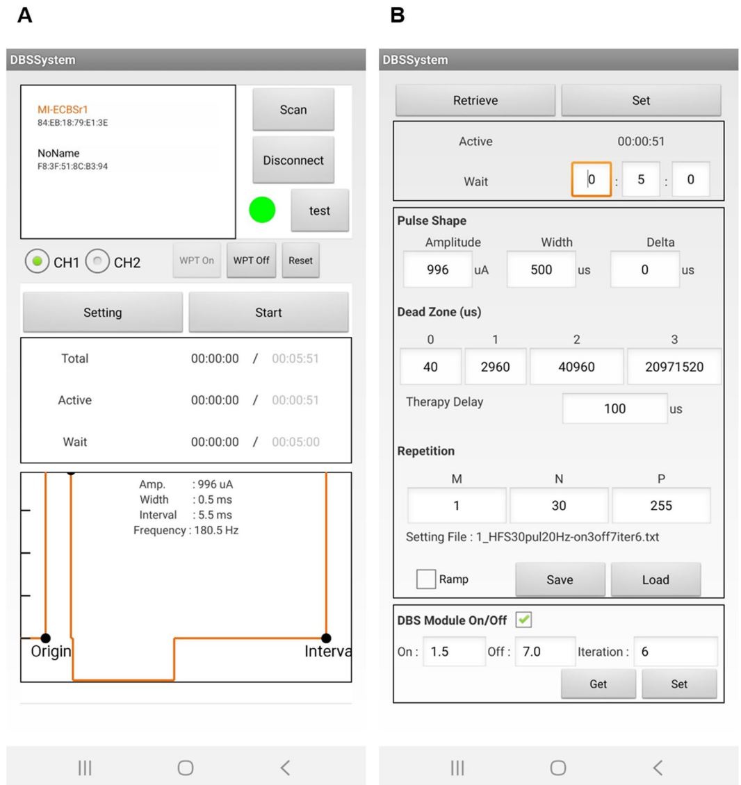
Figure 4. An illustration of the specified application of the smart device for the user interface. (A) the main window which the user can check a stimulation status and (B) the setting window which the user can adjust parameters.
