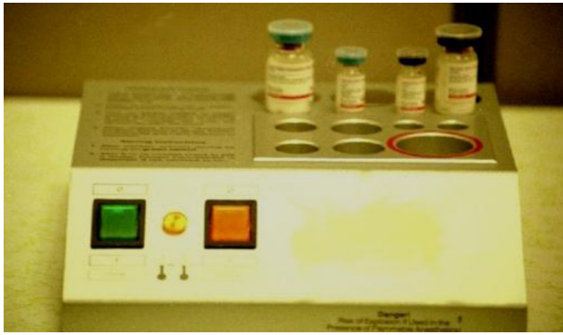
Figure 4 Manufacturer supplied Artiss device (Baxter, Westlake Village, CA) to facilitate dissolving freeze dried fibrinogen and thrombin powders in saline solutions.
