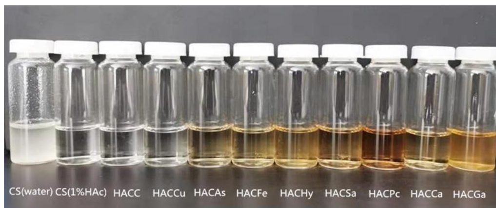
Figure 4. Solubility of chitosan derivatives (distilled water, 1 mg/mL) and chitosan (distilled water and 1% HAc).
