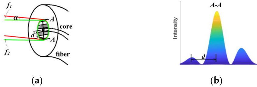
Figure 3. (a) The fiber without fiber coupler adopted for receiving the interference beams; (b) Intensity distribution diagram in the A–A cross-section.
