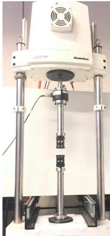
Figure 7. The experimental setup for tensile test on a Bone Bandid NiTi wire.
