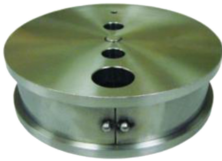
Figure 1. Expansion cell as per API RP 10B5.
