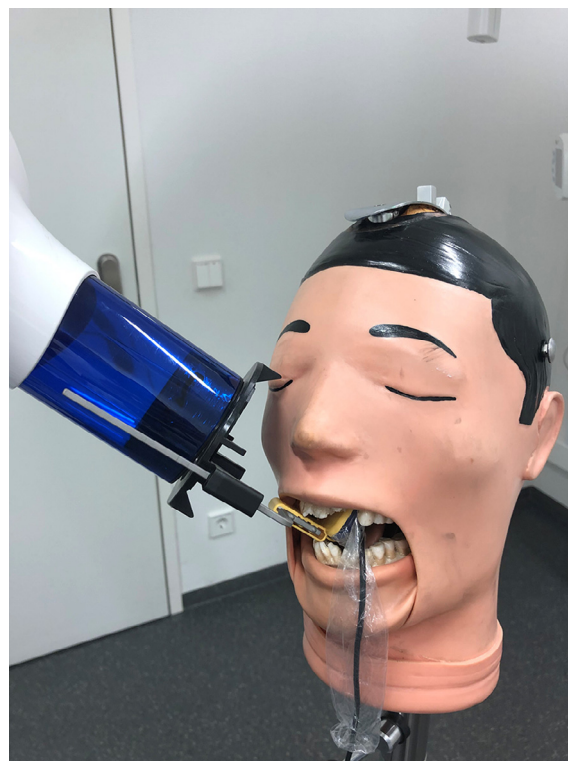
Fig. 2 Wall-mounted dental X-ray image acquisition of the upper right first molar using Heliodont Plus (Sirona Dental Systems, Bensheim, Germany).
