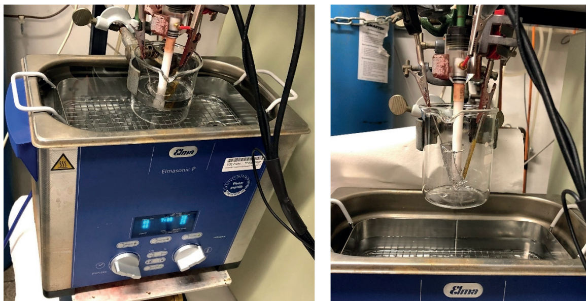
Figure 1. Photo of the experimental setup taken before carrying out the polarization experiments in the absence and presence of ultrasound a) and whilst performing the first activation procedure b).
