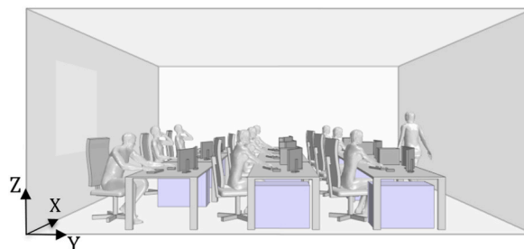
Fig. 1. Computational domain geometry. Measurements; X = 8.5 m, Y = 7 m and Z = 3.1 m. The classroom is maintained at a temperature of 21 °C and a relative humidity of 42% at constant atmospheric pressure.
