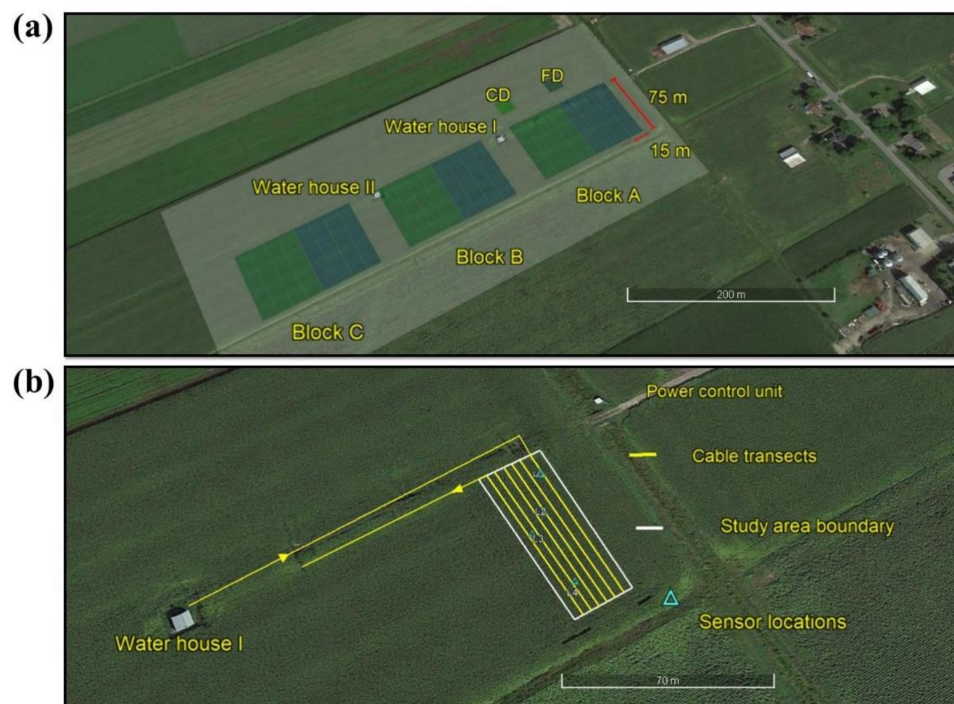
Figure 1. (a) Shows the study area which consists of three main blocks A, B and C. Blue and green rectangles within the main block are sub plots (15 × 75 m) of free drainage (FD) and controlled drainage (CD), respectively. Two water houses facilitate the measurement of drainage volume from each sub plot; (b) shows the fiber optic cable configuration in the field. Cable connected to the Distributed Temperature Sensing (DTS) instrument starts from the water house I and runs through two subplots at three depths (0.05, 0.10 and 0.20 m), blue rectangles show the locations of 5TE soil moisture sensors used for calibration and validation.
