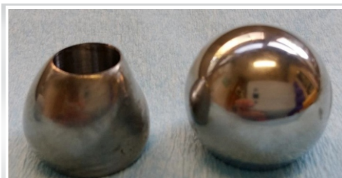
Figure 5: Picture of a retrieved worn CoCr femoral head (left) next to an unused femoral head of the same size (right). The femoral head was retrieved at the second revision of MoP bearing in 2013.
