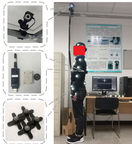
Figure 7. The overview of contrast tests between self-made and standard optical capture system.
