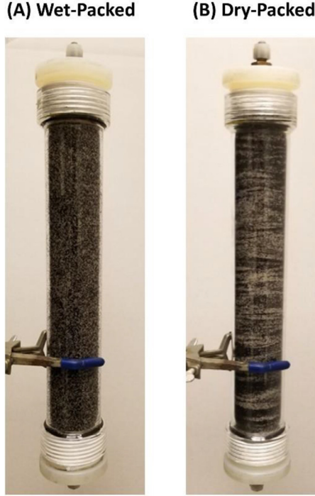
Fig. 2. A glass column ( L \times D = 30 \times 5 cm) filled with a sand and 4% biochar (g/g) with diameter of 0.5–0.595 mm packed under wet and dry ( \theta=20\% ) conditions.
