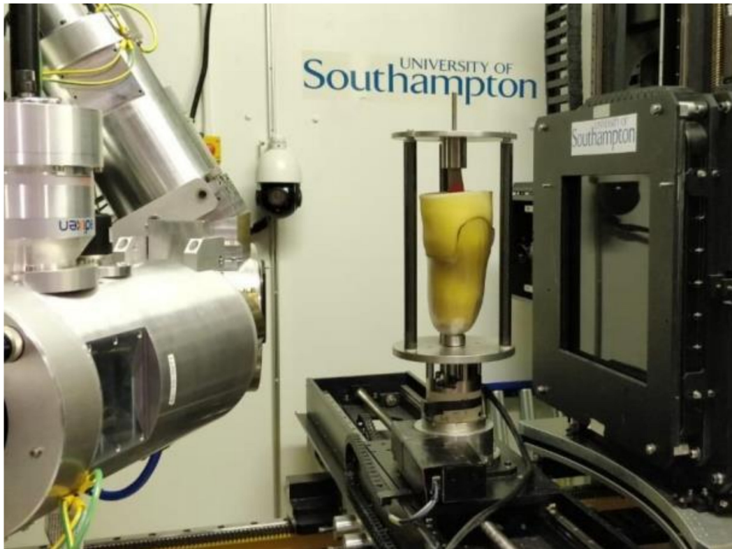
Figure 2. Analogue model and check socket mounted on the in situ loading rig inside the HUTCH microfocus CT scanner at \mu VIS X-ray Imaging Centre. Image shows X-ray source (left) and detector (right), with loading rig mounted on a rotate stage.
