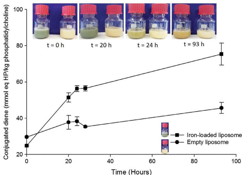
**Figure 1.** Conjugated diene (CD) hydroperoxide values in liposome suspensions (iron-loaded liposomes (■) or empty liposomes (●)), and macroscopic physical appearance of the suspensions during incubation at 40 °C (first images are always the empty liposomes, and second images the iron-loaded samples; the sample time is indicated underneath). Error bars represent standard deviations ( $n = 6$ ).
