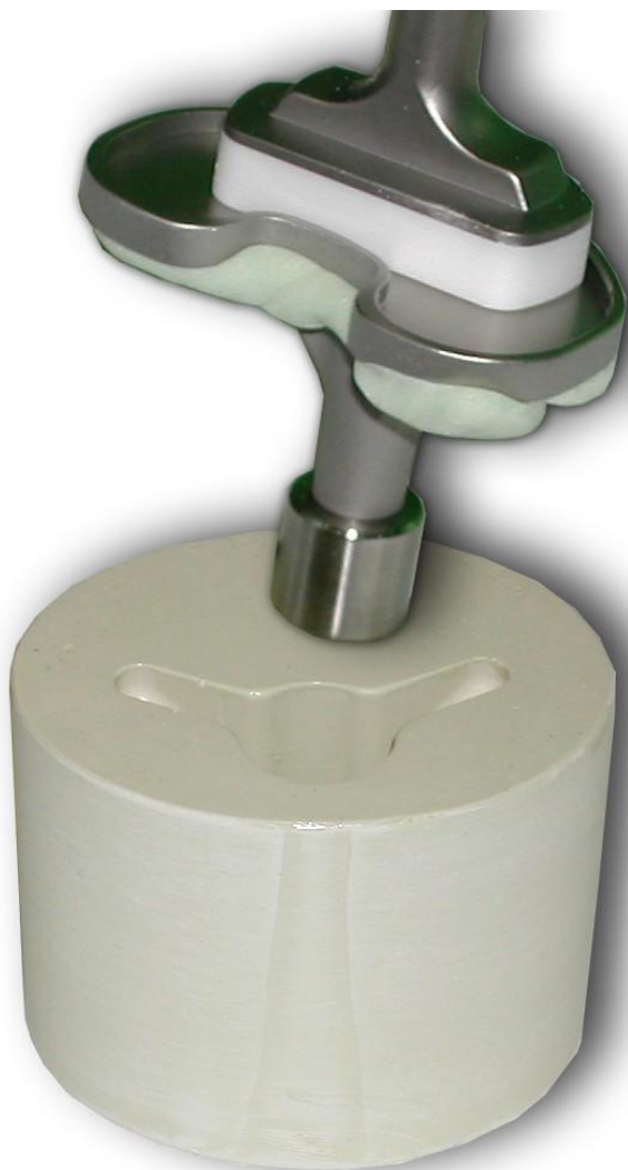
Figure 2 Tibial components ready for surface cementation onto the Technobones (below). Note that the central hole was machined such that there was no "press fit" between the TKA and the Technobones. This ensured maximum stress in the interface.
