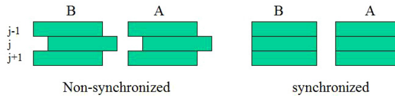
FIG. 1. Test fields with nonuniformly (left pair) or uniformly (right pair) extended MLC leaves. “A” and “B” indicate the left and right carriages. During dose delivery, the leaves move at the same speed and in the same direction, so the gaps (i.e., pattern) do not change. Six different gaps (5, 10, 15, 20, 25, 30 mm) and five different extensions (0, 5, 10, 15, 20 mm) were used in this study; thus, there were 30 test fields.
