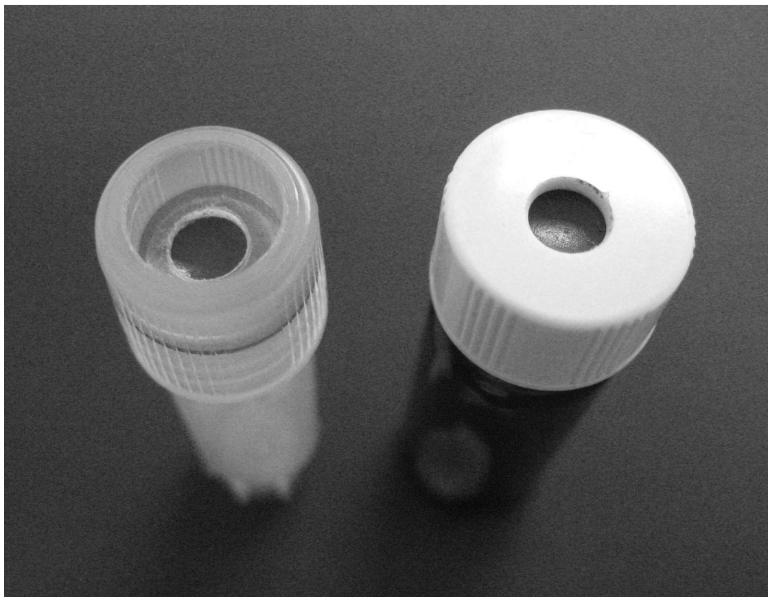
FIG 4 Reference material vials with pierceable silicone/Teflon septa.
