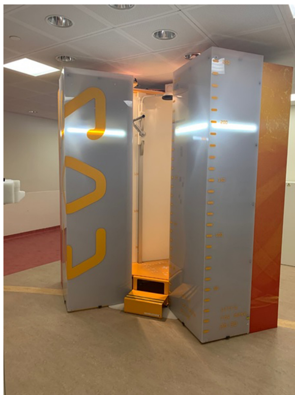
Figure 1. EOS System (EOS imaging, France) installed in our hospital. Patients step onto the central platform of the system where they stand whilst the image is acquired.
